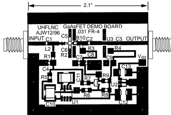
Figure 2. GaAsFET Demo Board showing component placement
